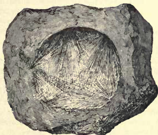
FIG. 67.—Drusy cavity in a lava, filled with zeolite which has crystallised in long slender needles.
